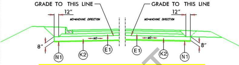
Class IV Subgrade Stabilization-Geotextile for Pavement Stabilization with ABC Base (New)
