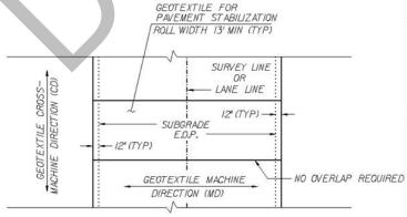
GEOTEXTILE FOR PAVEMENT STABILIZATION PLACEMENT (PLAN VIEW)
